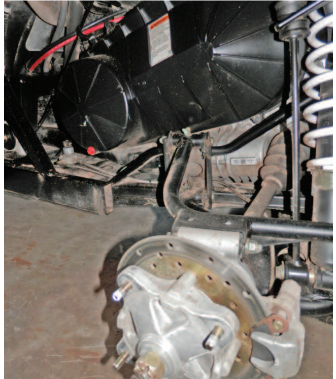
Access to the CVT cover is easy on the Polaris RZR 570. We removed the wheel for extra room.
