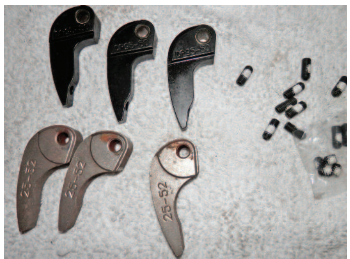
Notice the difference between the DALTON fly weights at the top, and the stock fly weights at the bottom. The weight inserts come in different sizes which can be changed based on your performance requirements.
